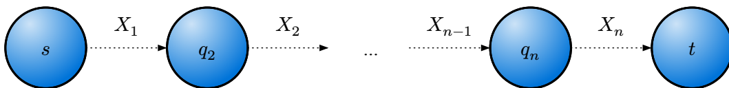
Figure 32: Sub-automaton created by calling connect , where the rhs is a sequence.
