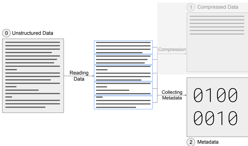
Figure 1: Preprocessing Procedure Scheme: The original unstructured text data (①) are read in chunks of similar sizes, all ending with a newline character. Metadata written to a separate metafile is collected for every chunk (②). Each chunk is compressed if the compression option is set, and the compressed data are written to a separate file (③).
