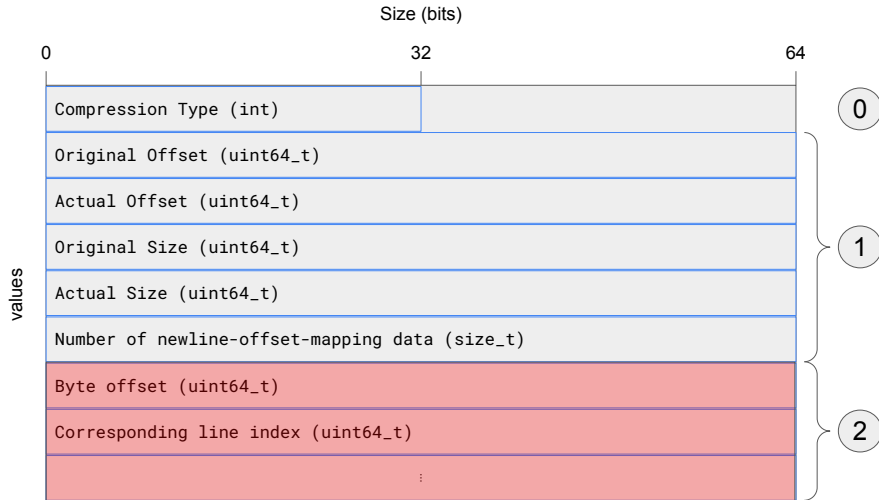
Figure 2: Metafile structure: The metadata are stored in a separate metafile in binary format. The metafile begins with an integer indicating the compression type (unknown: 0, None: 1, LZ4: 2, ZSTD: 3) of the data (①). Then, for every chunk, size and position information and the number of collected line index mapping data are stored (②). The line index mapping data are stored for each chunk separately (③).
