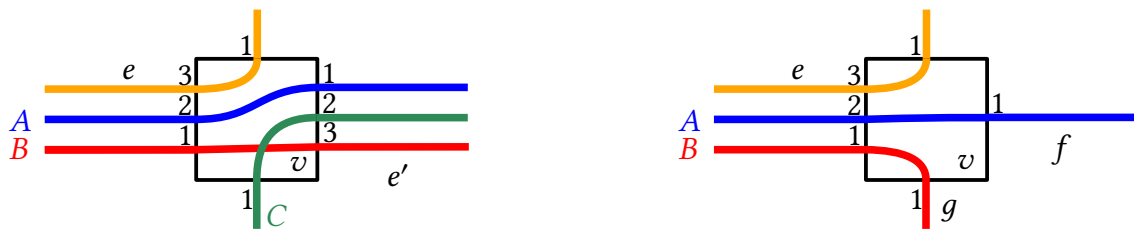
Figure 4.7: Left: Lines A and B are separated in v by C. Right: The branching of A and B into two different edges f and g does not count as a separation.
