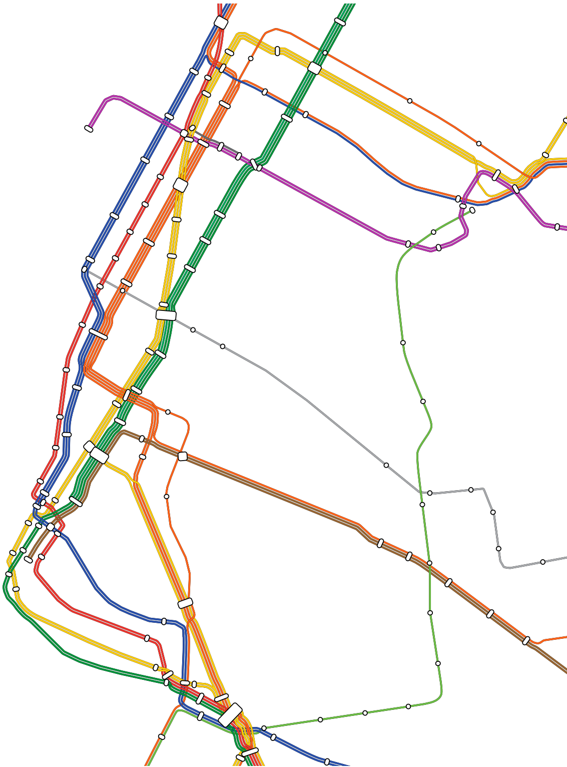
Figure 4.45: Excerpt from a line-ordering optimized rendering of the New York subway network, optimized by our ILP in 0.6s. Line graph generated by our pipeline described so far, rendered using the approach from Chapter 6 by the transitmap tool (Chapter 7).
