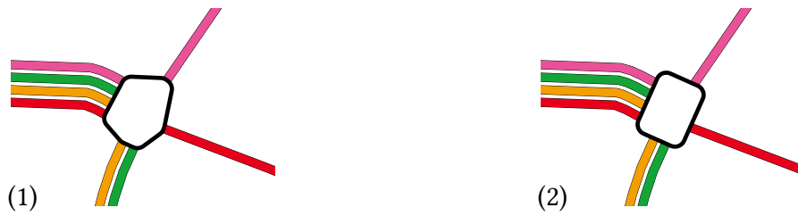
Figure 6.9: (1) Station marker rendered using the convex hull of the node fronts (2) Station marker rendered using the oriented bounding box of the node fronts.
