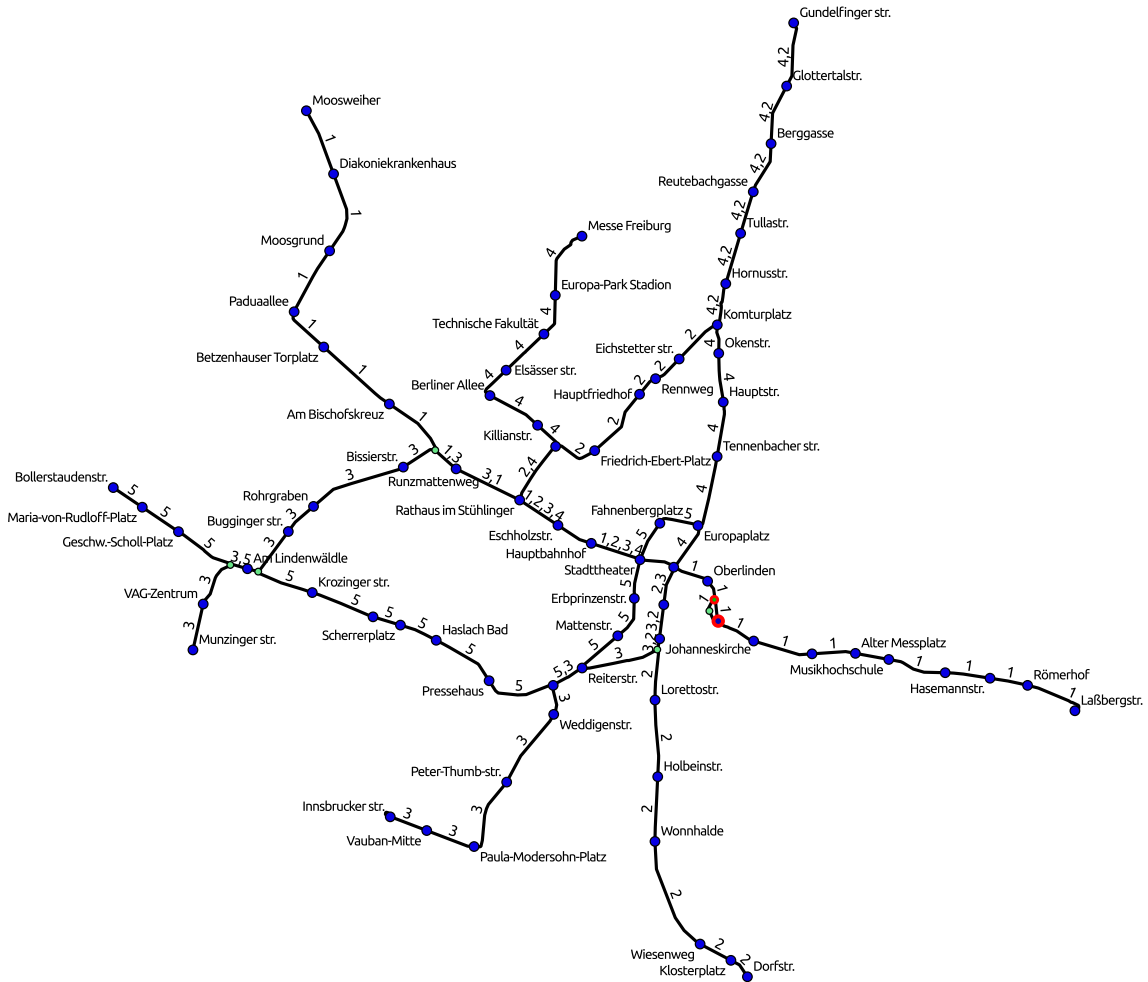
Figure 3.15: Line graph for the 2022 tram network of Freiburg, created from raw schedule data using the approach described in this chapter. The input schedule data was first map-matched with our approach from Chapter 2. The merge threshold was set to \hat{d} = 40 m. Stations are given in blue, non-station nodes in green, and nodes with a red outline have inferred turn restrictions. Not all station and line labels are shown.
