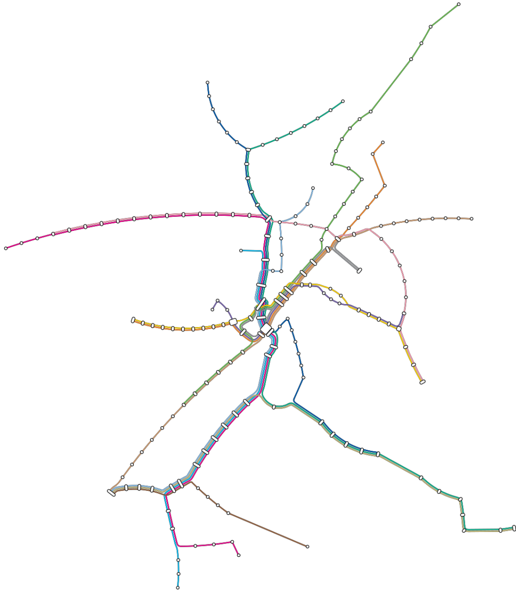
Figure 7.4: Curvilinear transit map of the 2016 Stuttgart light rail network generated using our pipeline and the schematization approach by Fink et al. [58]. The approach was implemented as a drop-in replacement for octi as part of a student project.
